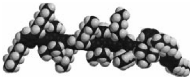
Figure 2. Representation of a polymer chain of 3e . The calculation was performed with the MM2 force-field by utilizing Spartan Pro. Note the irregular conformational and rotational positions of the bulky side chains and the likewise bulky CpCo units in this polymer.
